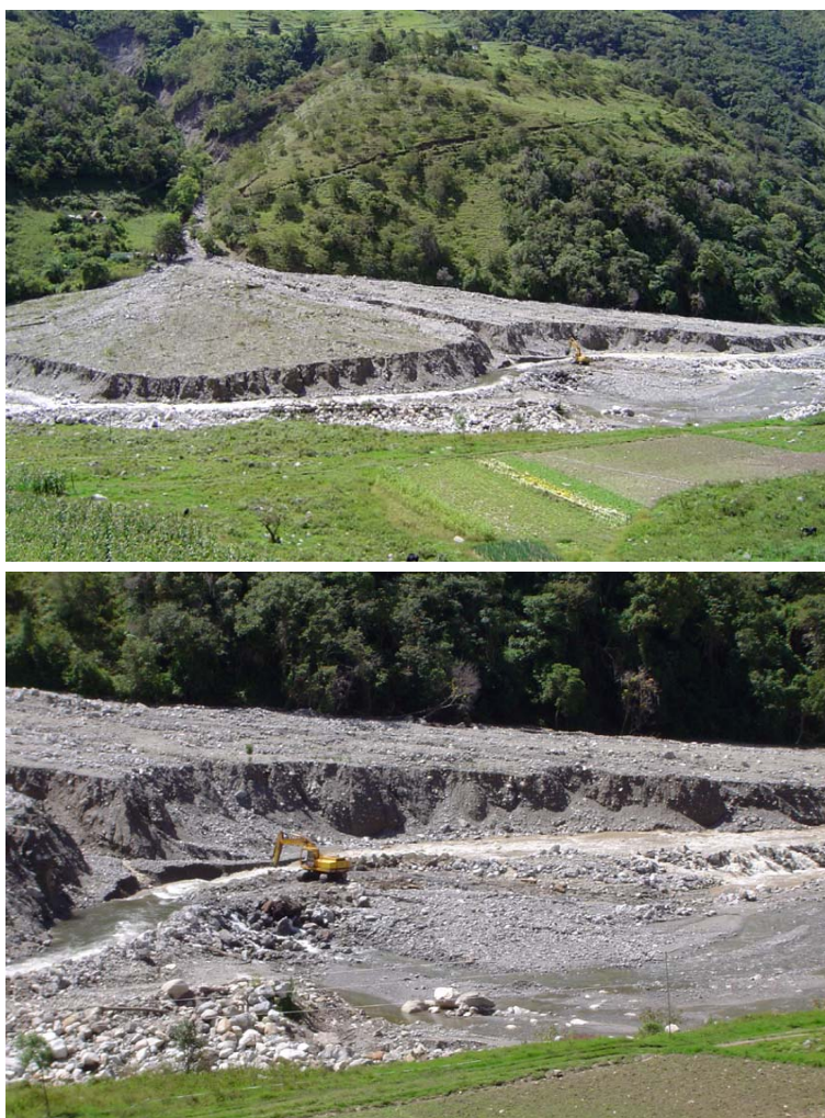
Figure 10. Extraction of sand and rocks in Chama River for the construction industry, Mérida State,
